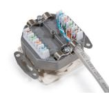
Place the wires correctly according to T568A Fasten the cables with metal holder in place Cover up with the metal cover. of the shielding.
